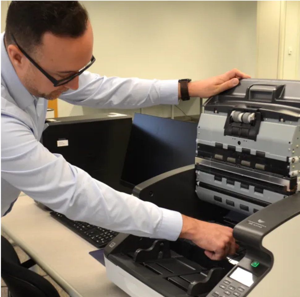
Oakland County Director of Elections Joe Rozell shows spots inside one ballot-counting machine where glass is regularly cleaned to minimize false anomalies. Peg McNichol / MEDIA NEWS GROUP
