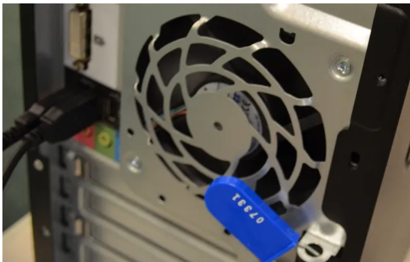
Election equipment is secured with numbered plastic cable ties or with plastic-and-metal locks that break when removed. Peg McNichol / MEDIA NEWS GROUP
